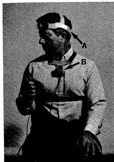
Fig. 1. Subject with electromagnetic sensors in place. A) Sensor and B) Source unit.
