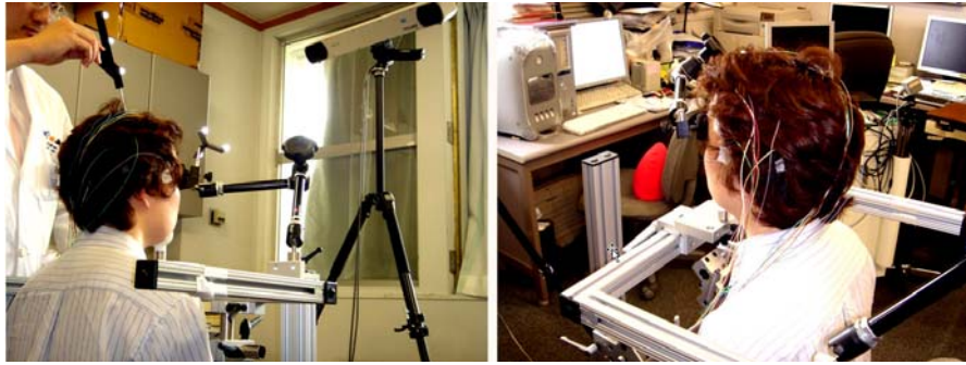
Figure 1. Frameless stereotactic image guidance system (a real-time MRI-navigator system, Brainsight ®)
